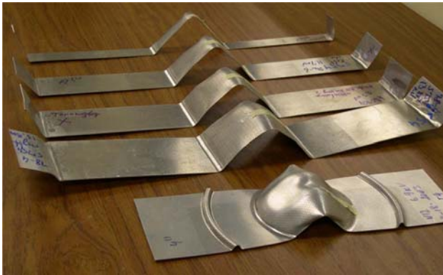
Fig. 8 Samples after testing formability with pulsed electromagnetic field driving samples into the dies with an open round or rectangular window
