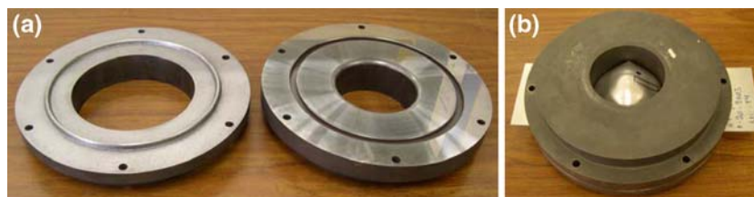
Fig. 5 The die for forming into an open round window with the draw bead: (a) in open position; (b) in closed position
